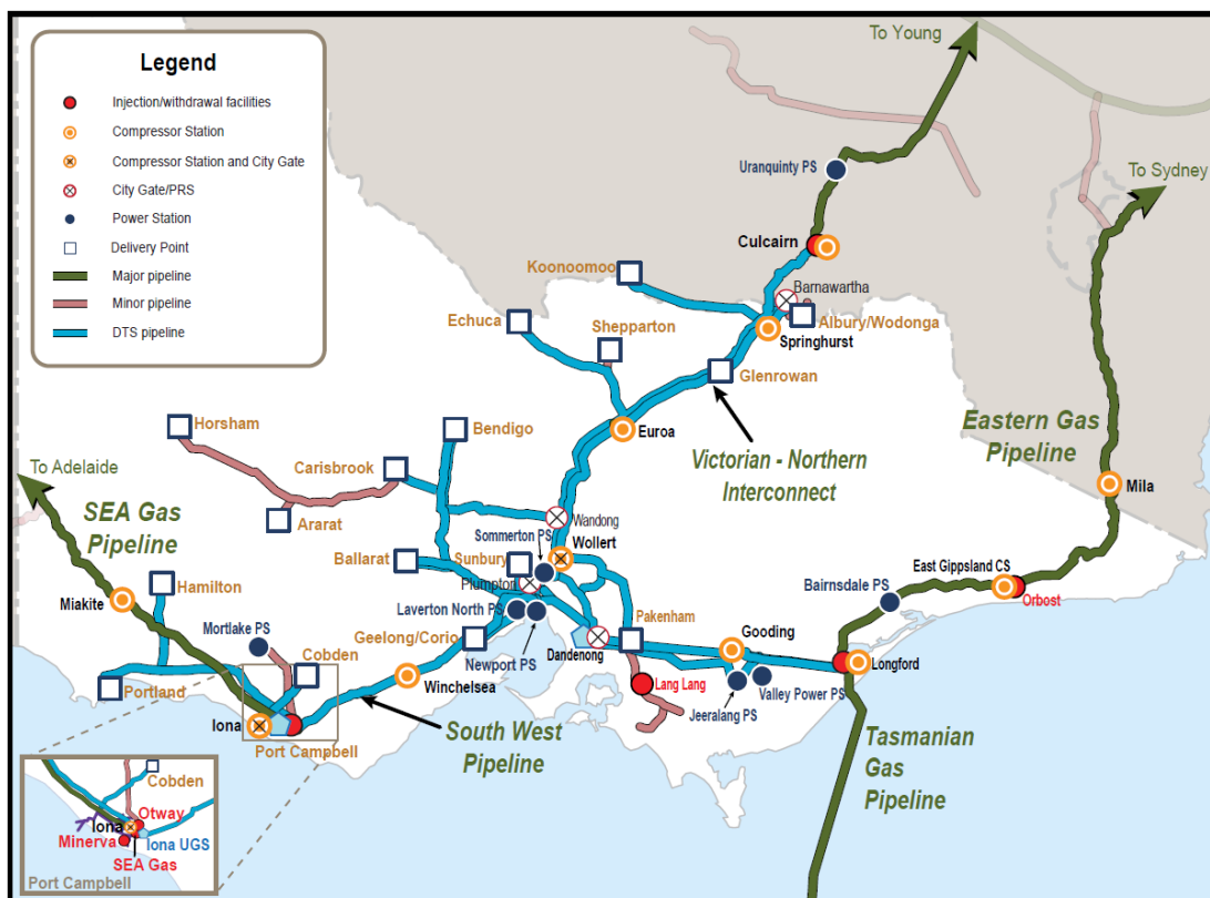
Figure 3 The Victorian Declared Transmission System
