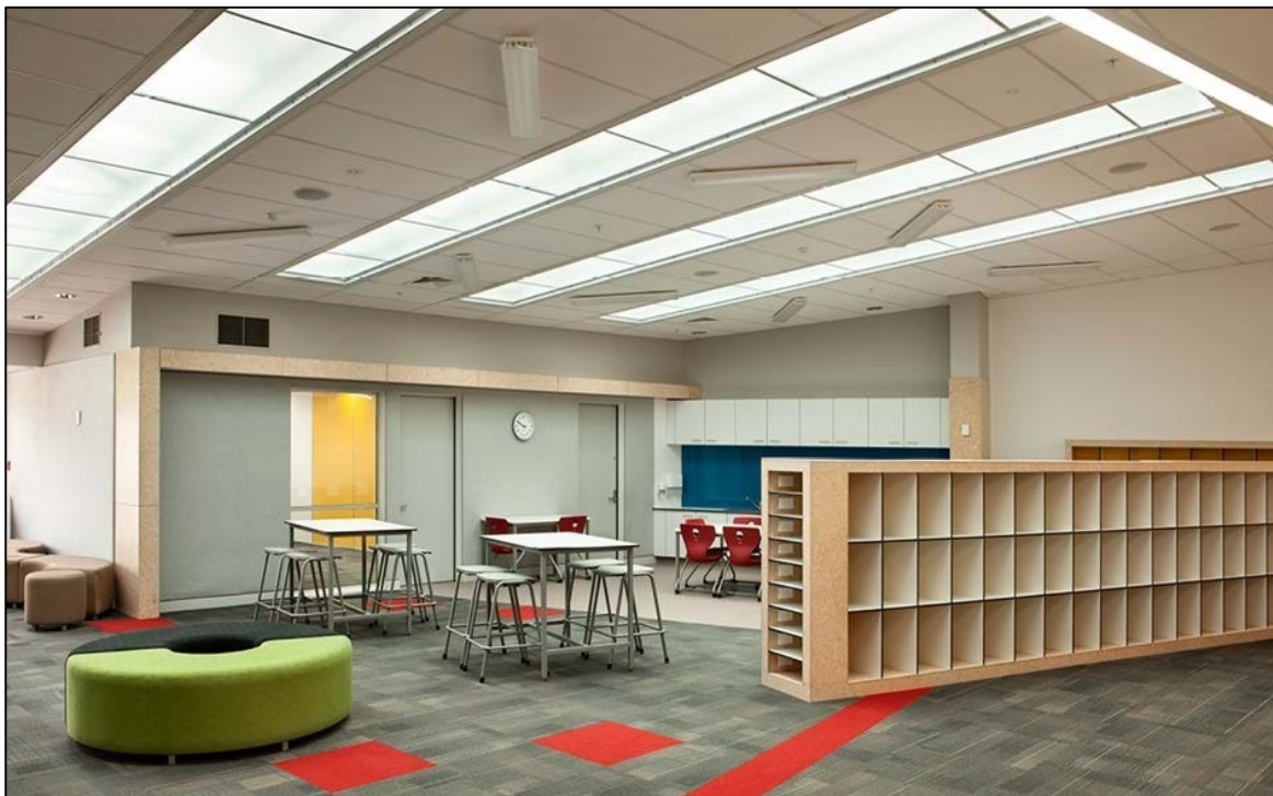
Figure 23: Extensive natural roof light system with more limited side lighting maintains good daylight levels, but with reduced outside awareness
