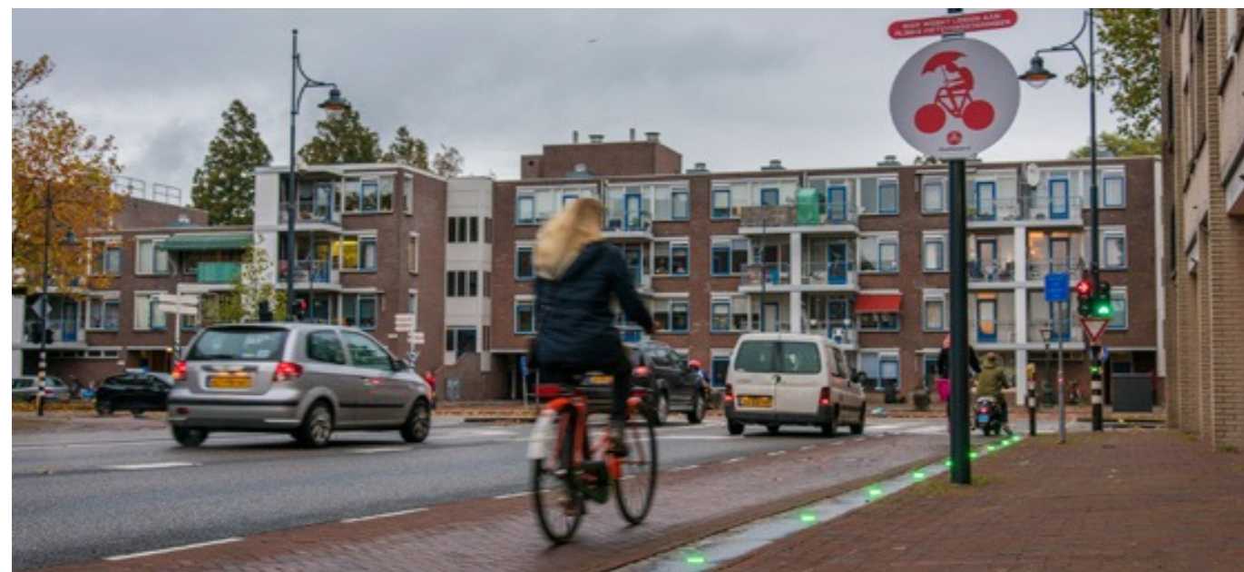
Figure 12. A ‘Green Wave’ in the Netherlands using green lights to indicate synchronised signals [Source: CROW Fietsberaad (2016)].
