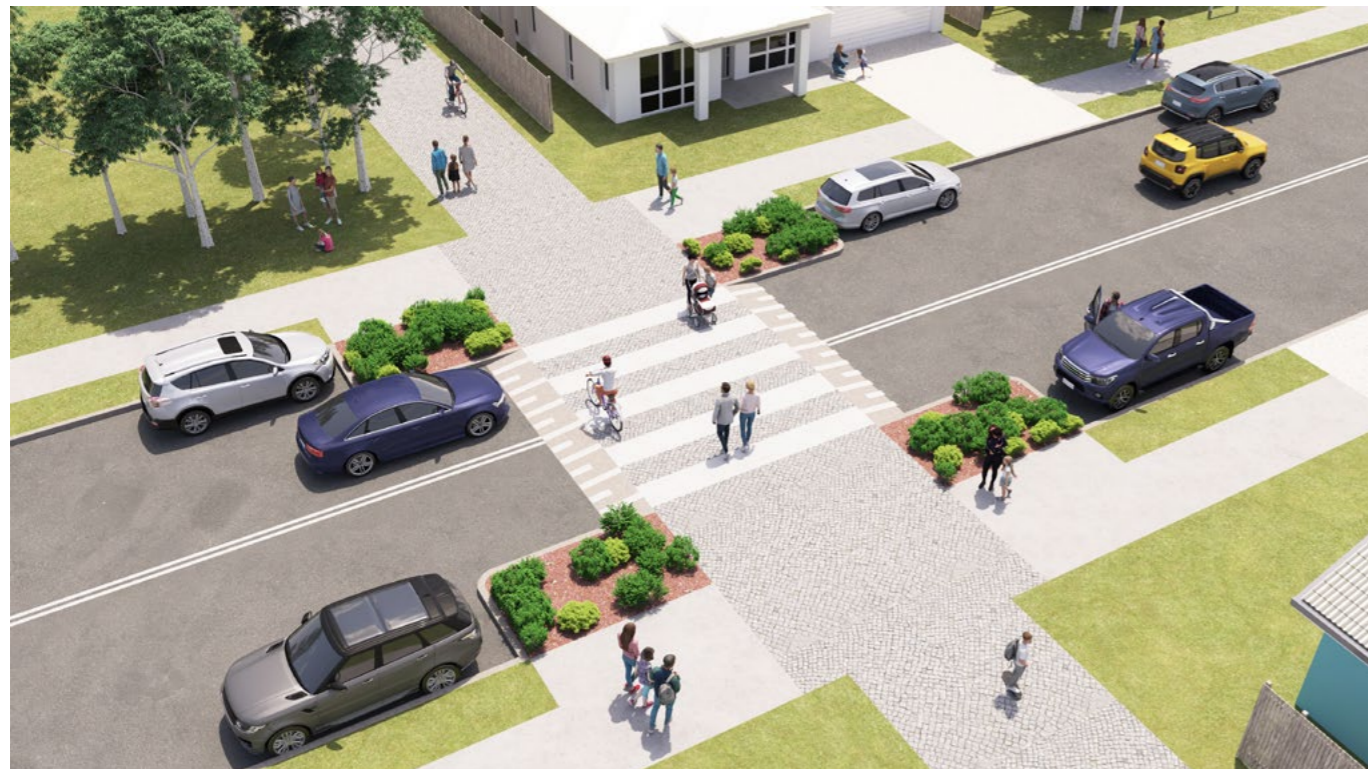
Figure 15. Local path network intersection with a local street, prioritising walking and cycling movements .
