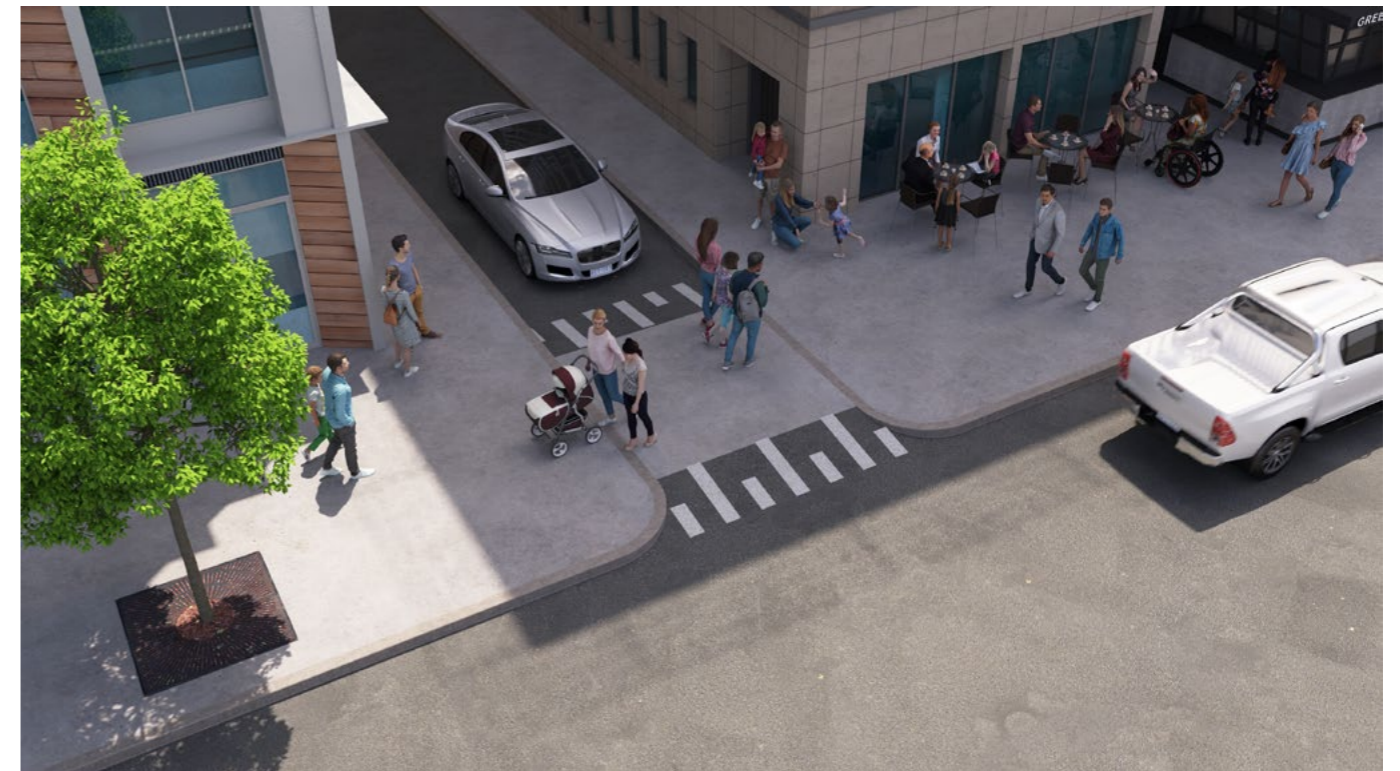
Figure 14. Priority crossing over driveways [adapted from the Urban Street and Road Design Guide (Auckland, 2022) ].
