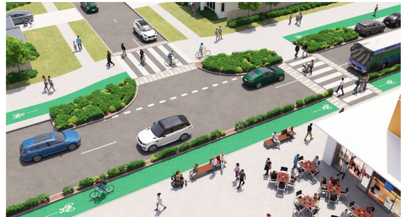
Figure 17. Bent out path where a local road meets a collector road [adapted from Cycleway Design Toolbox. Designing for cycling and micromobility (Transport for NSW, 2020)].
