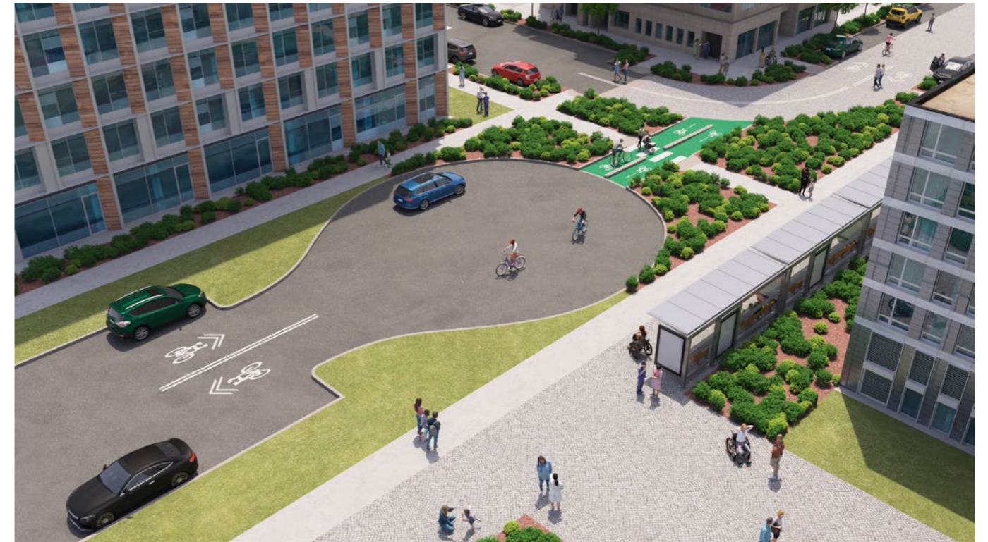
Figure 21. Modified T-intersection to restrict motor vehicle traffic and allow walking and cycling to filter through [adapted from Cycleway Design Toolbox. Designing for cycling and micromobility (Transport for NSW, 2020) ].
