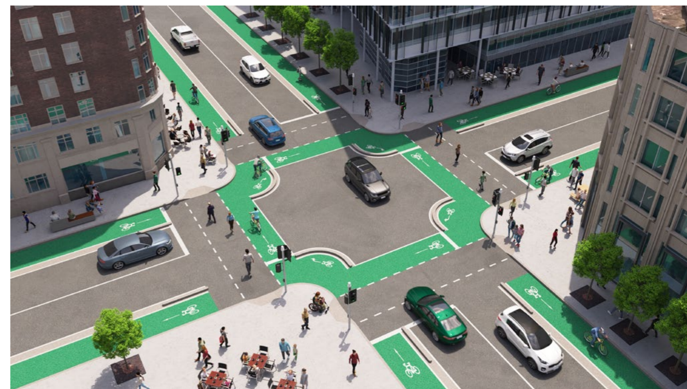
Figure 23. Collector to collector intersection where bicycle routes are present in both directions, [adapted from Cycleway Design Toolbox. Designing for cycling and micromobility (Transport for NSW, 2020)].
