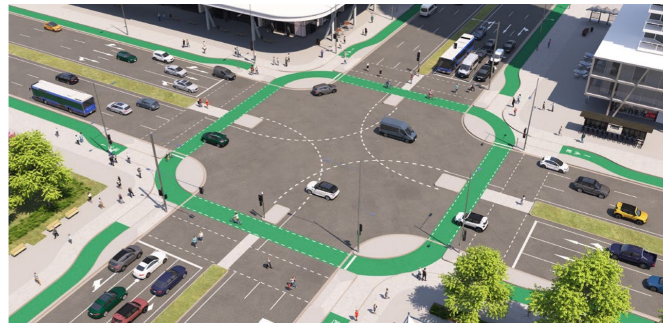
Figure 25. Arterial to arterial intersection with priority to active users [adapted from the Urban Street and Road Design Guide (Auckland, 2022)].
