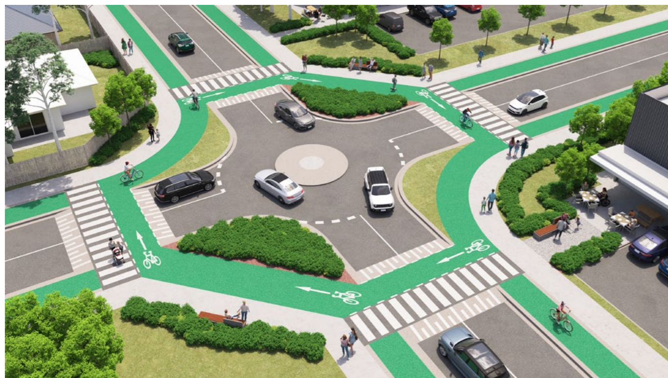
Figure 24. Tightened kerb radii slows turning traffic and increases visibility between road and path users (adapted from Cycleway Design Toolbox. Designing for cycling and micromobility [Transport for NSW, 2020]).
