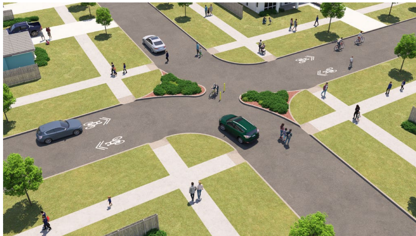
Figure 20. Treatment to reduce the number of intersections for cars and retain permeability for walking and cycling [adapted from the Urban Street and Road Design Guide (Auckland, 2022) ].
