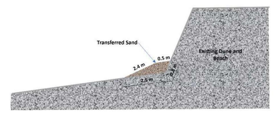
Figure 5-6. Approximate dimensions for the placement of 1 m<sup>3</sup>/linear metre.
