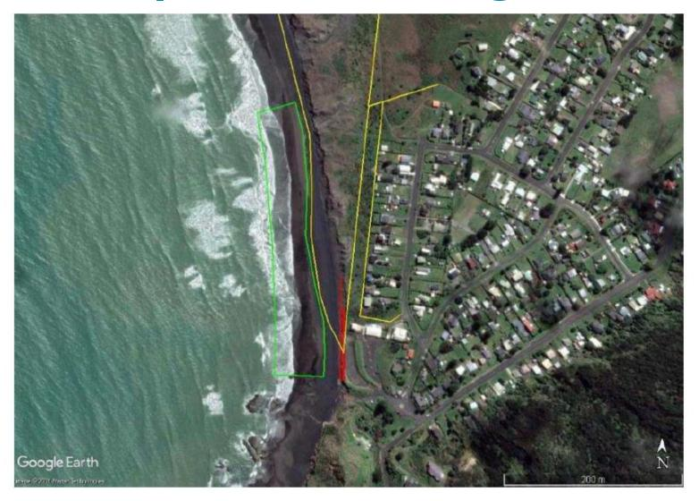
Figure 5-5. The most vulnerable 150 m of southern Sunset Beach (thin red line), and the 100 m (thick red line) where 100 m³ of sand should be distributed as a buffer zone until larger volumes are available. The yellow lines denote the approximate boundaries of the DoC area and the Outstanding Landscape area to the west of the 20 m wide WDC esplanade reserve. The green box delineates the recommended borrow site, which is approximately 400 m long by 70 m wide (i.e., ~28,000 m²).
