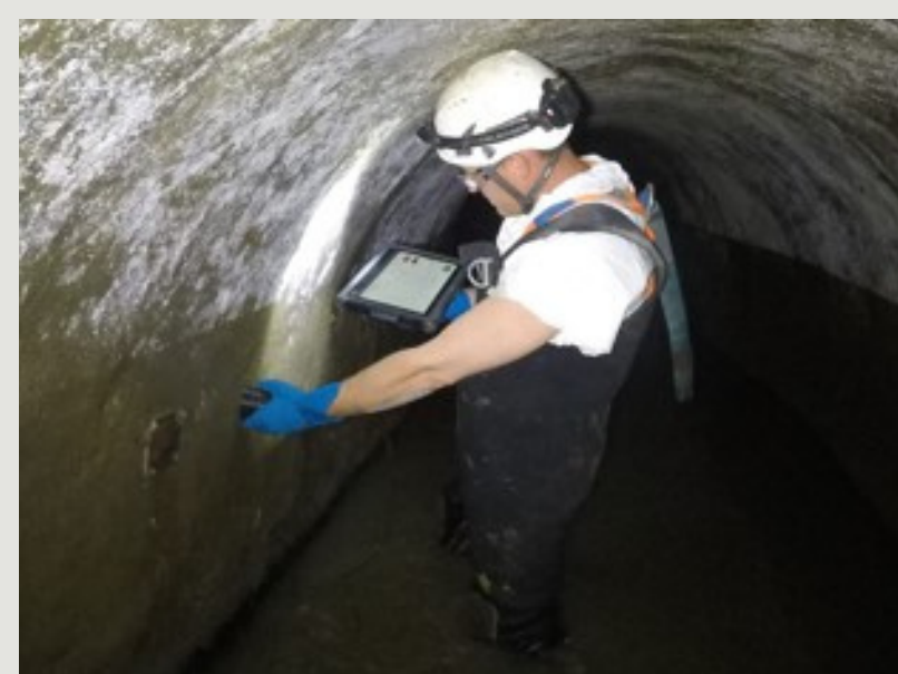
CAC/Geopolymer thickness sensor field test
