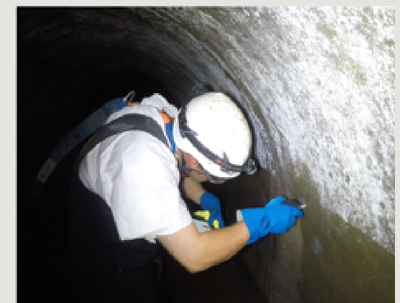
Acid permeation sensor field test
