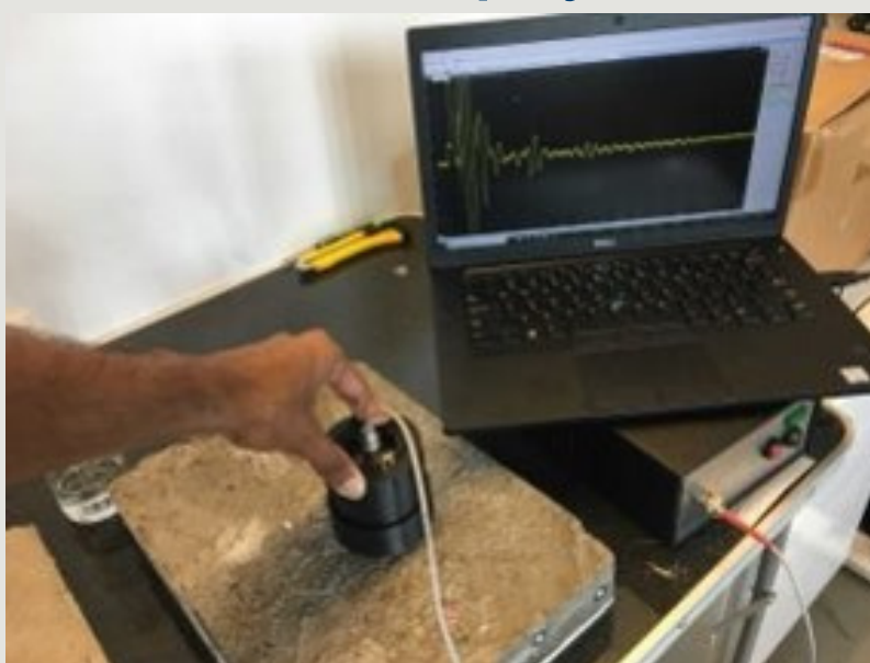
CAC/Geopolymer thickness sensor lab test
