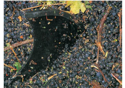
Piece of a fish plate from harvester.
