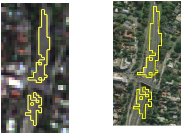
Figure 2c: False positive - highway verge identified as synthetic turf on Sentinel 2 imagery (left) and higher resolution satellite imagery (right)
