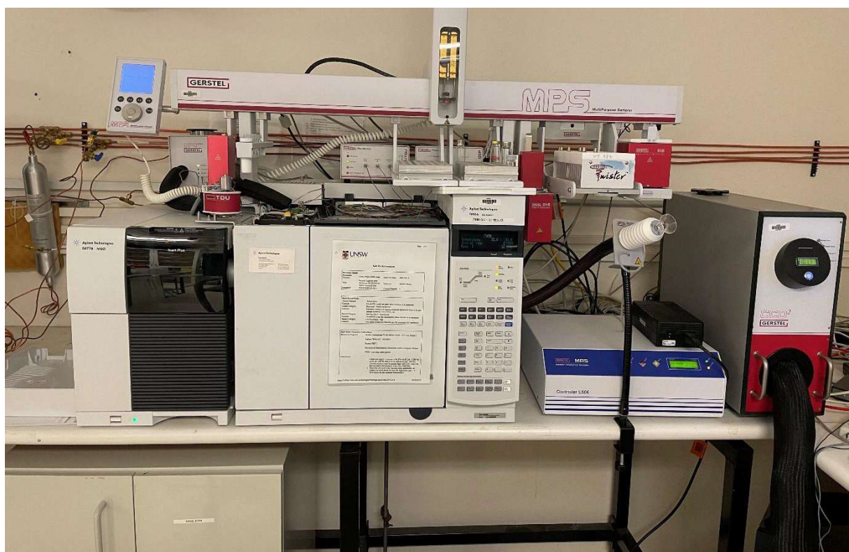
Figure 5. Example of a GC-MS/O setup. Samples are first placed in the left-hand side of the device where the GC separates the sample into its constituents, and then subsequently detected by MS. Note the olfactory detection port on the right-hand side for use by the
