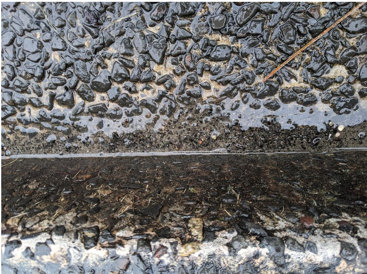
Figure 11: SBR Infill (upper half of photo) located in a gutter. SBR infill was mobilised over several metres of grass verge from a Sydney ST field.
