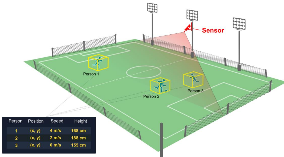
Figure 1: Illustration of an ideal sport field sensing solution. A sensor is placed at a specified location to identify players on the field, with additional information, such as speed and height, being displayed on a dashboard.
