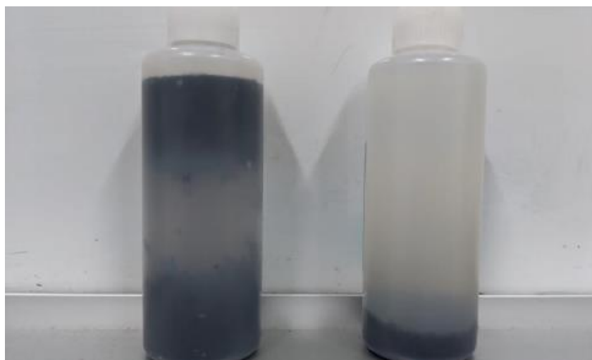
Figure 8: Rubber infill material in water after one hour (left) and one week (right)
