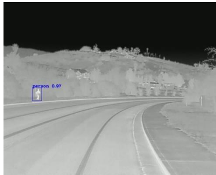
Figure 6: A thermal image taken from inside a car. Human bodies appear as bright objects even in difficult conditions, and can be identified (at a basic level) using machine learning. Image adapted from [8].
