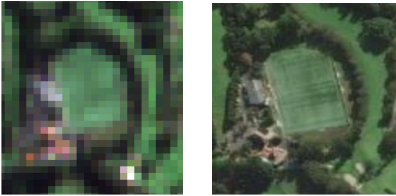
Figure 2b: False negative - synthetic turf field not identified by algorithm on Sentinel 2 imagery (left) and higher resolution satellite imagery (right)
