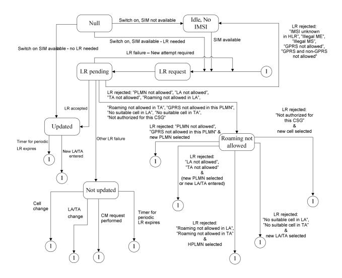
NOTE 1: Whenever the MS goes to connected mode and then returns to idle mode again the MS selects appropriate state.
