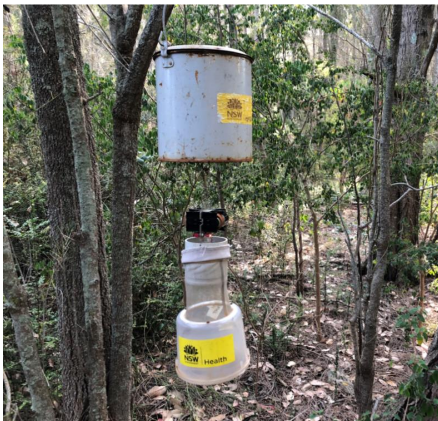
Figure 3. An example of the carbon dioxide-baited “Encephalitis Virus Surveillance” traps used to survey adult mosquito populations at five locations within the Northern Beaches local government area, December 2019 through May 2020.
