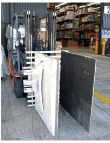
Figure 7: Using suitable equipment to unload such as a fork lift truck with grabs.
