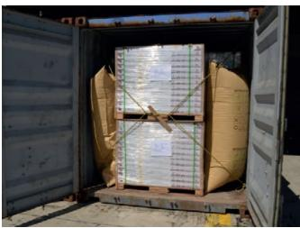
Figure 4: Bulky items packed using crates, wrapping, dunnage bags and strapping.
