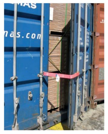
Figure 3: Use restraints to ensure doors can be opened safely.
