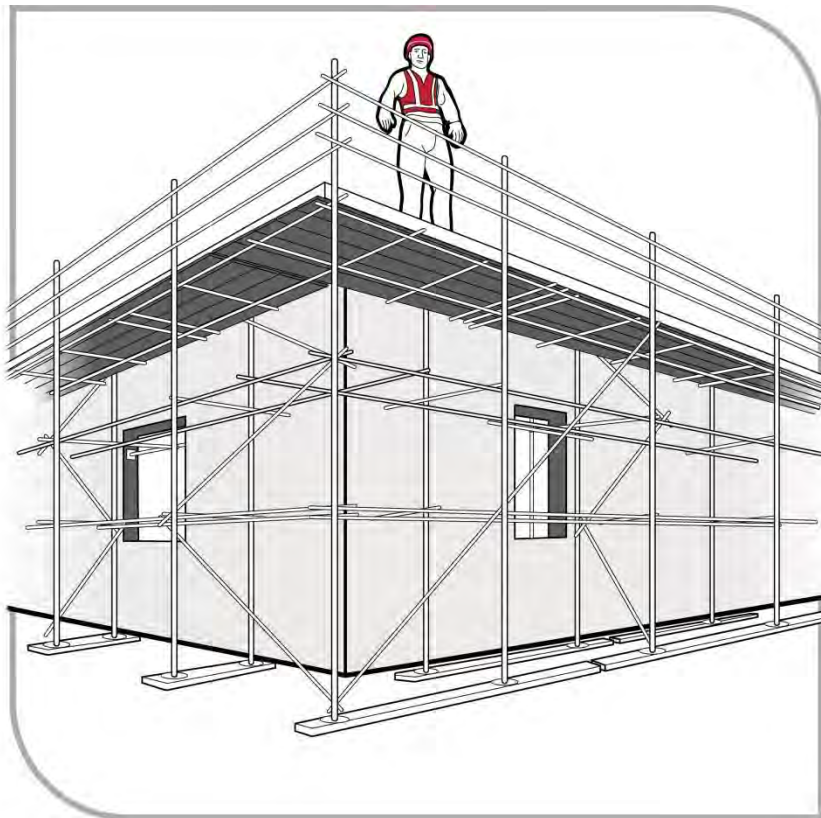
Figure 7 Perimeter scaffold with fully decked working platform, guardrails, mid-rails and toe-boards
