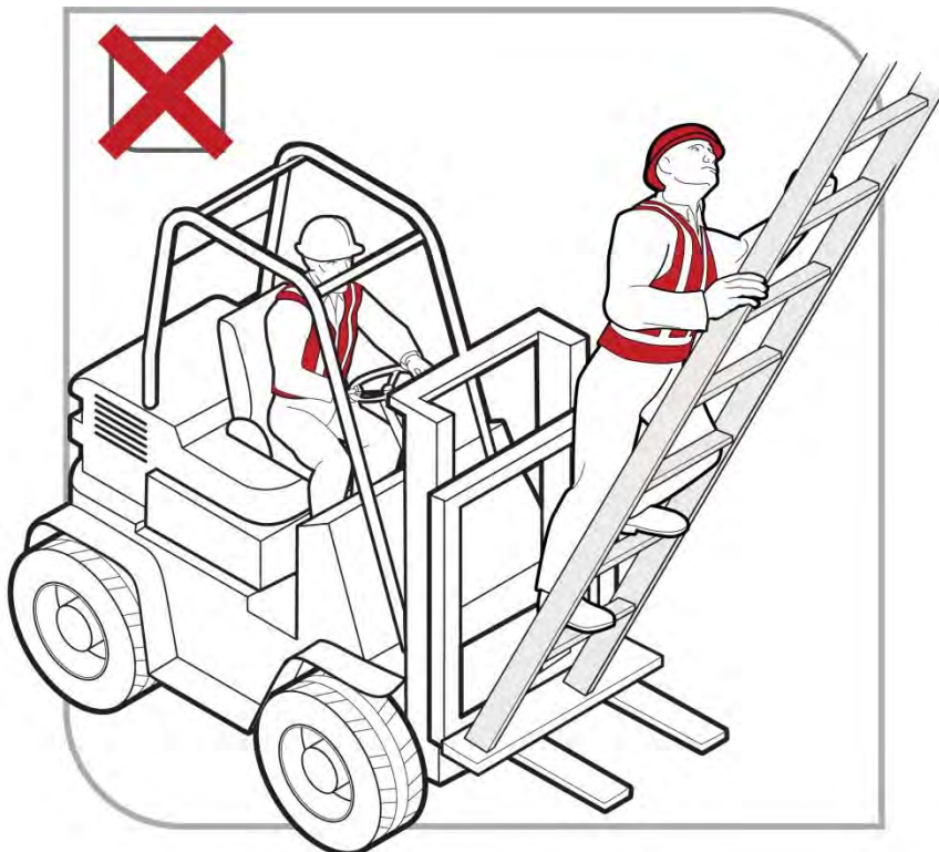
Figure 14 Using a forklift as a working platform or to gain extra height by standing on the tynes or a pallet is an unacceptable practice
