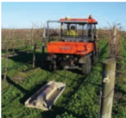
Figure 3.12a. EM38 being used to determine potential salinity variation in a vineyard
