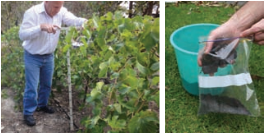
Figure 4.2. Soil sampling by auger along the vine row and packaging in plastic bags to send to laboratory
