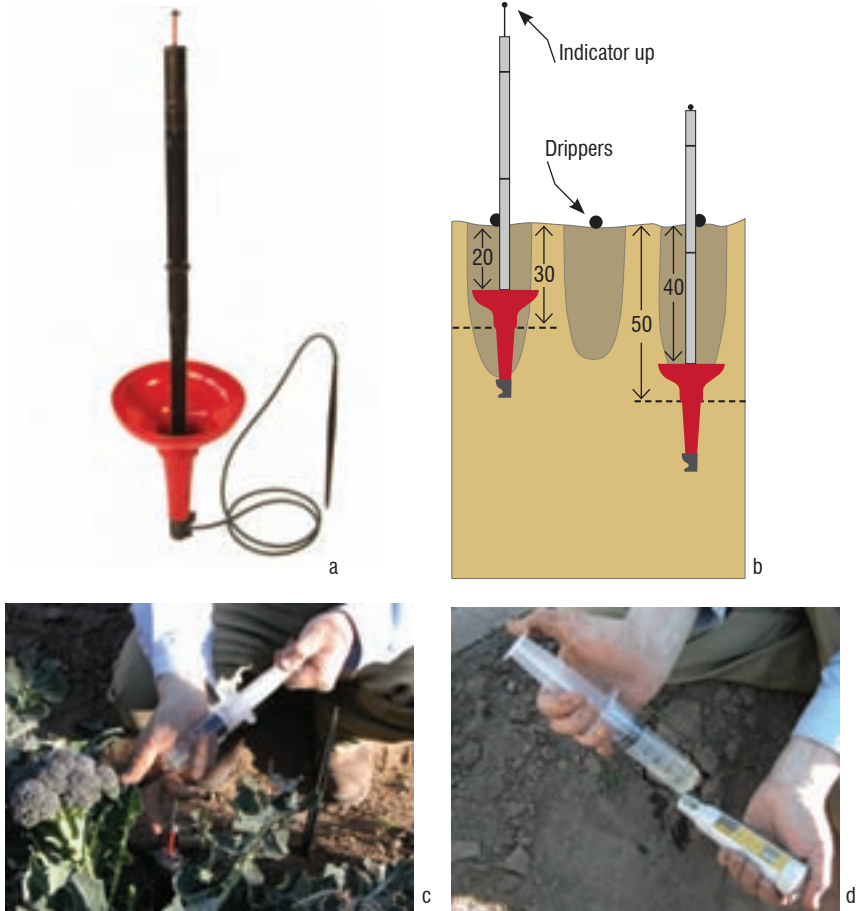
Figure 4.4. a) The FullStop wetting front detector, b) suggested placement of the FullStop wetting front detectors beneath drippers, c) extracting the soil water sample, and d) testing a soil water sample extracted from the FullStop for salts. (Source: CSIRO)
