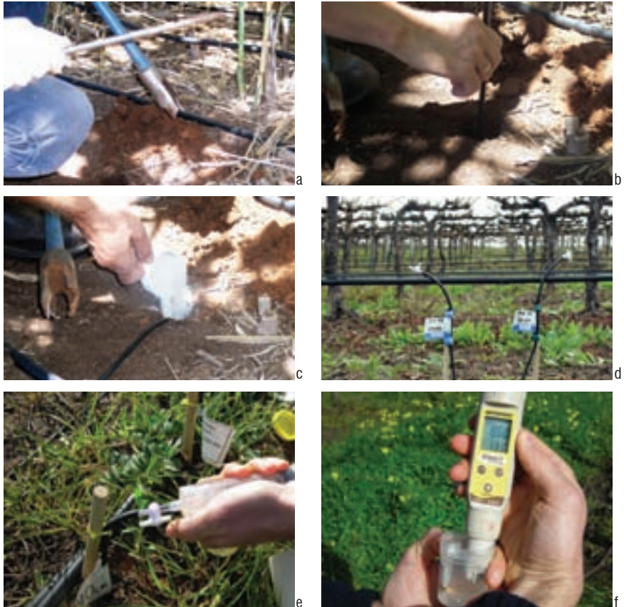
Figure 4.8. SoluSAMPLER™ installation and measurement a) augering hole to desired depth, b) insertion of the SoluSAMPLER™, c) placement of a bentonite plug to prevent preferential flow, d) tagged extractor tubes, e) application of suction to collect soil water sample, and f) measurement of the soil water sample using an EC meter. (Source: SARDI)
